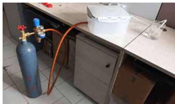
Indigenously developed Carbon dioxide based euthanising setup for rodent samples.
